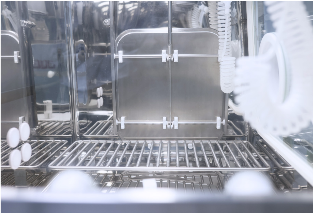
Isolator technology for weighing API hormones | Veropharm - Abbott | Russia
