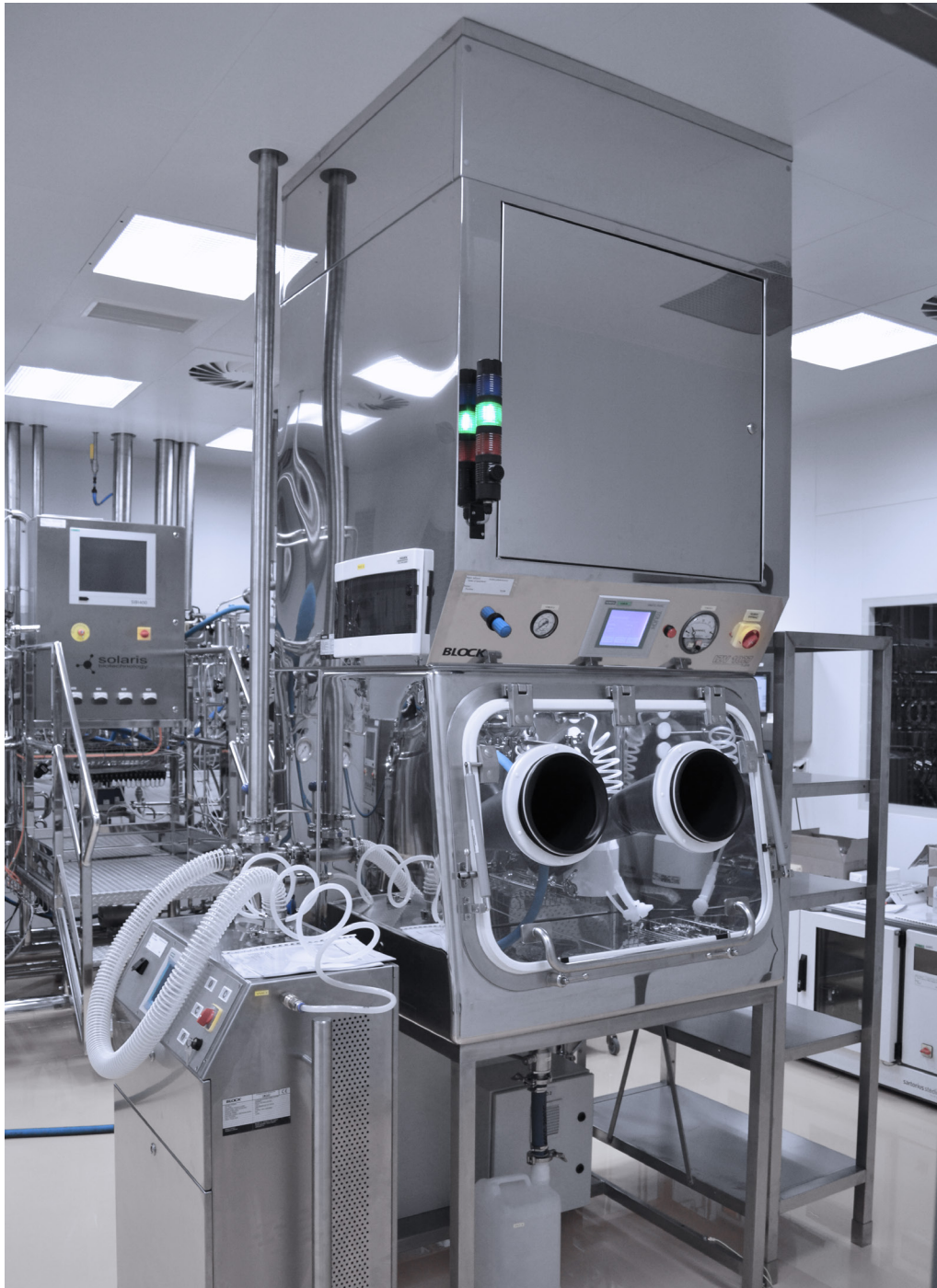
Isolator for handling viruses and infectious substances | Bioveta, a.s.; Ivanovice na Hané | Czech Republic
