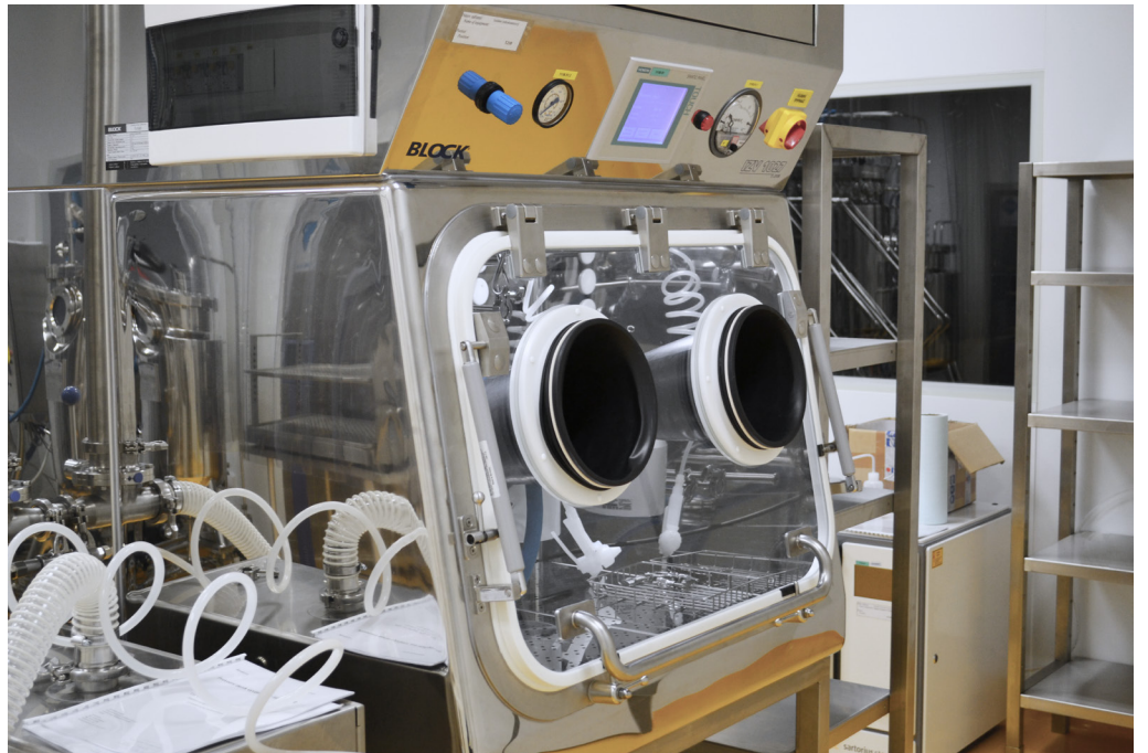
Isolator for handling viruses and infectious substances | Bioveta, a.s.; Ivanovice na Hané | Czech Republic
