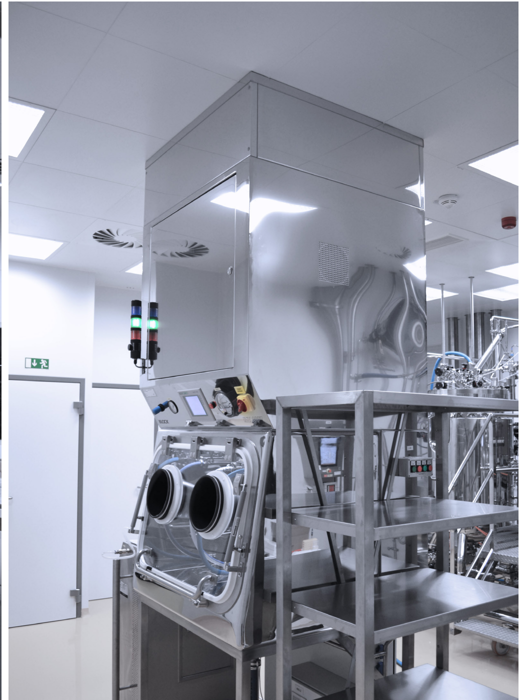
Isolator for handling viruses and infectious substances | Bioveta, a.s.; Ivanovice na Hané | Czech Republic
