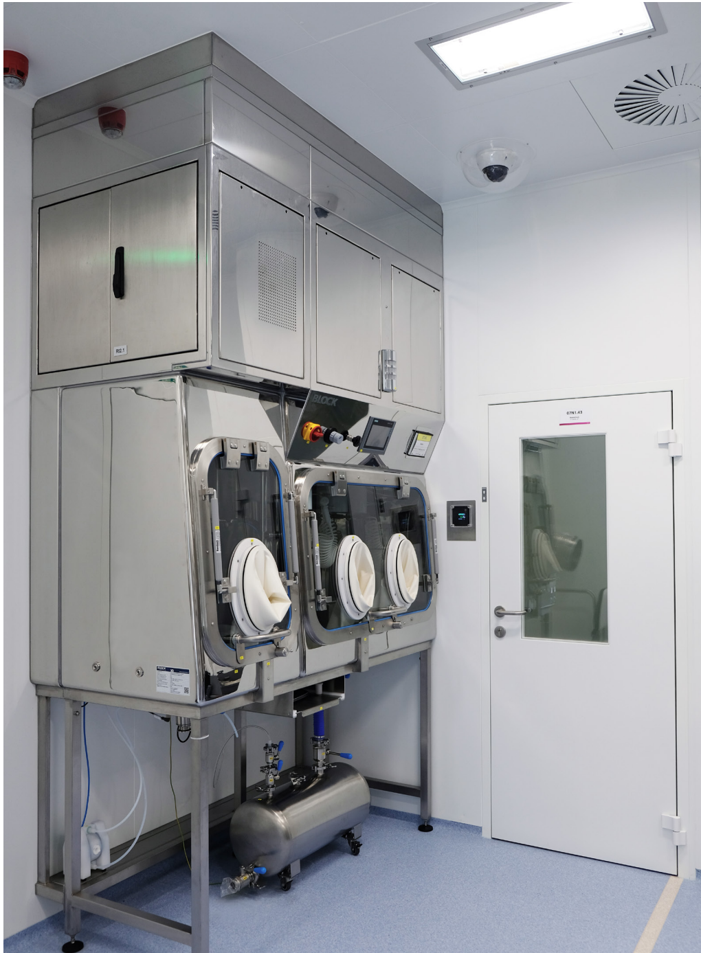
Isolator for Spray Dryer | Synthon, s.r.o. | Czech Republic
