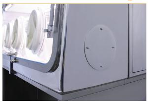
The site for the RTP is placed on the chamber's right wall. Option to integrate an RTP alpha port and beta container for sterile transfer of materials.
