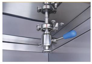
For outlet of liquid waste originating from sterility testing. Connection to a collecting tank or central waste.
