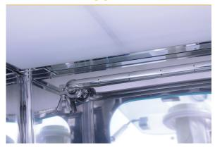
This isolator can be sterilised using hydrogen peroxide vapours. A uniform distribution of vapour is achieved using a perforated pipe installed through the whole length of the chamber.
