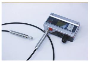
This sensor is very important for controlling process decontamination. Rotronic is an accurate and high-quality product, resistant to hydrogen peroxide vapours.
