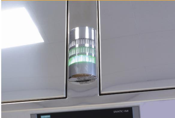
A beacon light and an acoustic alarm providing a quick audible and visual assessment of operation and failure states for the user.
