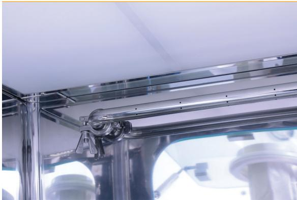
This isolator can be sterilised using hydrogen peroxide vapours. A uniform distribution of vapour is achieved using a perforated pipe installed through the whole length of the chamber.
