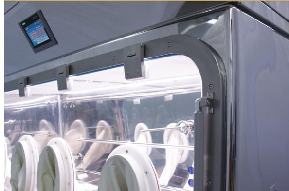
Inflatable sealing safety glass fitted with sleeved flanges and sensors for monitoring safe window closure. A gas spring is used for easy opening.
