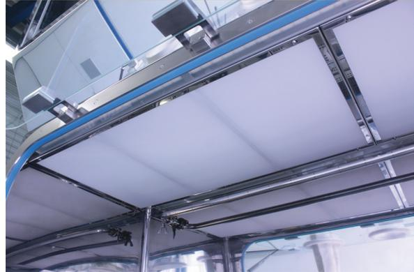
The chamber ceiling is fitted with a laminar frame for producing laminar flow, and includes built-in LED lights. Inlet HEPA filters are situated above the laminar frame.
