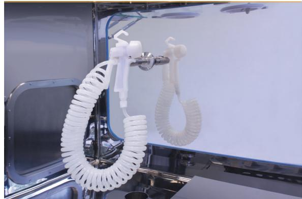
Easy cleaning of the isolator is made possible with an installed spray gun. It operates with two media and is controlled by a valve via the HMI panel. For washing, the chamber is connected to water piping and dried by switching over to compressed air.
