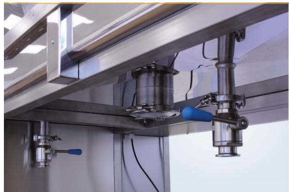
Tri-clamp connection for an optional connection to the building waste pipe system or to add a collecting container.
