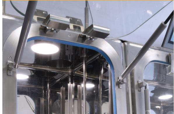
Inflatable sealing, safety glass fitted with sleeved flanges. Sensors for monitoring safe window closure. A gas spring assists with easy opening.
