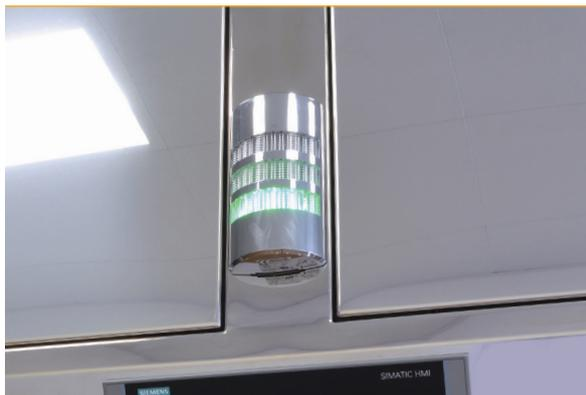
A beacon light and an acoustic alarm providing a quick audible and visual assessment of operational and failure states for the user.
