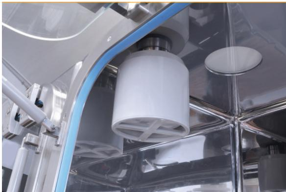
Highly efficient H14 filters remove ultra-fine impurities from the air in the inlet and the outlet.
