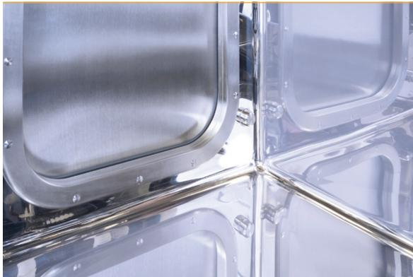
Rounded corners and highly polished surfaces allow for easy cleaning of the chamber. The chambers are precision-welded which guarantees their leak tightness.
