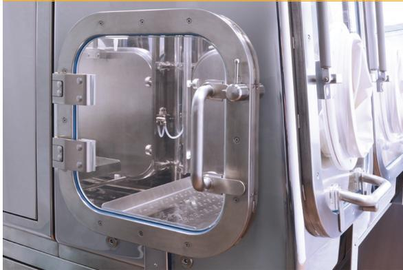
The door allows for material transfer from the chamber to the surroundings or from the chamber to other equipment (e.g. a fume hood). The hinged door is operated with the help of a door latching mechanism. The door is made from AISI 316L stainless steel, safety glass and silicone sealant.
